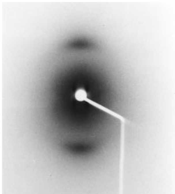
Figure 6. X-ray diffraction pattern recorded at room temperature for a melt-extruded fiber of P12-9NPd.
